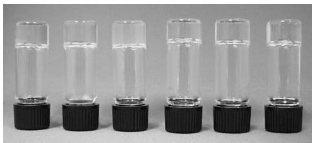
Figure 2. Gels (5 mg/1 mL) of 1 -citronellol, 1 -rose oil, 1 -lavender oil, 12-HOSA -limonene, 12-HOSA -orange oil, and 12-HOSA -lemon oil.
